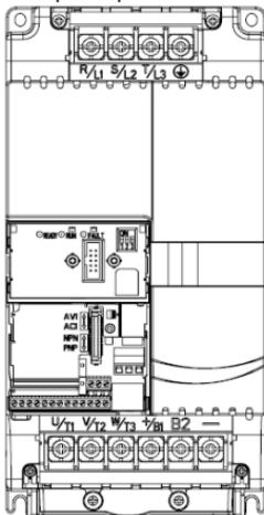
Силовые терминалы: R/L1, S/L2, T/L3, U/T1, V/T2, W/T3,
